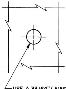
USE A 33/64" (.5156) DIA. DRILL. BORE HALFWAY THROUGH DOOR ON ONE SIDE ONLY. (PLUG TO BE FORCE-FIT INTO DOOR.)
