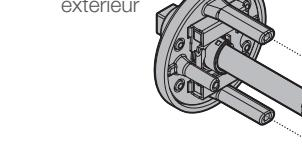
Press latch bolt to install exterior chassis.
