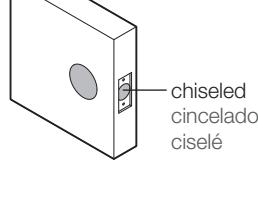
If door edge is NOT chiseled, install drive-in collar.
