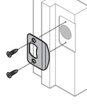
Close door and test latch operation. If latch is loose in the strike, adjust strike tab so it grips the latch bolt better when the door is closed.
