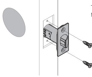
The slant of the latch bolt faces in the direction that the door closes.
