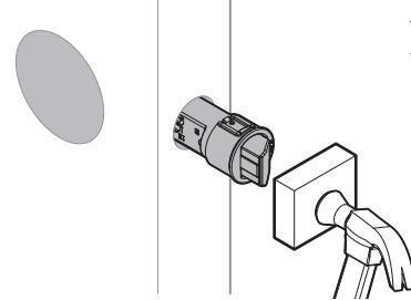
The slant of the latch bolt faces in the direction that the door closes.
