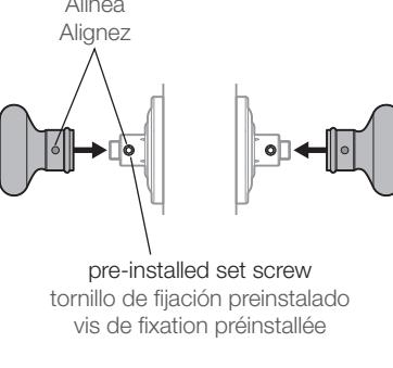
Tighten pre-installed set screws.
