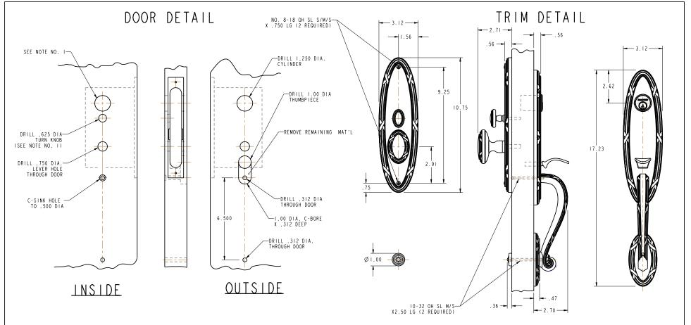
DRILL A Ø 1.250 CYLINDER HOLE INSTEAD, USING SAME CENTER LINE AS OUTSIDE CYLINDER HOLE.
