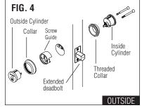
slot of inside cylinder with notch in threaded collar. Keeping tailpiece vertical and curved toward the right side of hole, insert inside cylinder with threaded collar into the deadbolt. Attach cylinders using two #10-32 x 2-1/4" flat head machine screws. Tighten screws. Do not insert key during this procedure. (Fig.4)
