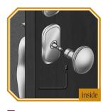
7 Slide knob/lever onto dummy inside adapter with set screw hole down and toward hinges until it is flush with rosette. Insert set screw and tighten with
