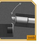
2 (Arial View) Alignment of Latch Strikeplate: Curved edge of latch strikeplate should face curved side of
