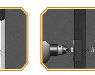
**5** Very carefully drill (A)  $2\frac{1}{8}$ " hole into one side of door face until drill bit starts to protrude on opposite side. Important: Drill perpendicularly (at a 90°
