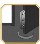
Pull door toward you to check if it's level. Observe contact of door to jam and make sure it's level. Adjust if
