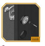
2 Insert dummy cylinder through dummy cylinder collar and into outside of door. From inside, insert retaining screw through lock washer and locating plate, then scre into dummy cylinder.
