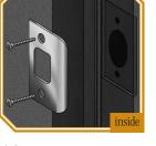
10 For Latch Strikeplate: Insert dustbox into hole, add strikeplate, and secure by inserting #8 x ¾" wood screws into pilot holes.
