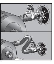
When fully inflated, seal valve by pushing in with pump nozzle. This will seal the internal yellow stopper and keep air from escaping while closing cap. Gently twist adapter sleeve to right while backing pump out of valve.
