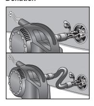
Remove adapter nozzle from inflation end and attach to deflation side of pump. Repeat same steps as inflation. This will draw the air out quickly.
