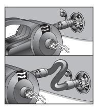
Attach adapter nozzle to inflation end of pump. Insert pump and turn on.
