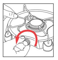
Adjust flame with burner valve.
