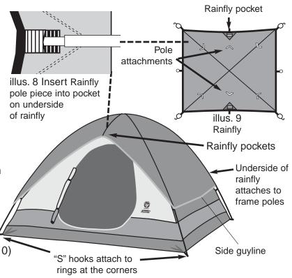
illus. 10 Completed tent with rainfly. Note where rainfly pole pockets, pin & rings, and frame ties are located
