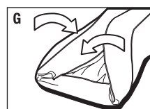
Deflating - Push flapper valve open into locked position
