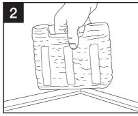
Place the pump chamber snugly in the selected corner.
