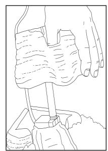
Place the outlet on pump and then attach it to the waterfall unit. Tip-Lubricate the pump outlet with water to ease assembly. Place the waterfall unit on top of the pump chamber. Make sure the pump lies in vertically in the chamber. Note-Make sure the waterfall sits securely on top of pump chamber. Do not
