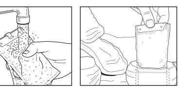
Remove the filter cartridges from the packaging. Rinse them under cold tap water to remove carbon dust, and place them into the slot of each chamber. Push the cartridge until it hits the bottom and place lids to close chambers.
