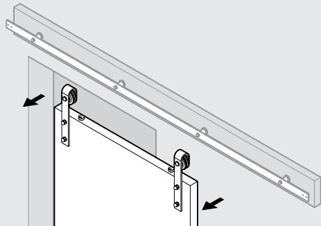
**B Remove the set of fasteners that were preventing the door stop from moving into position.**
