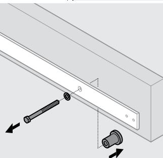
**C Slide the door stop onto the track, past the hole where the fasteners were removed.**
