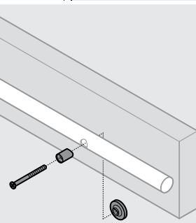
**C Slide the door stop onto the track, past the hole where the fasteners were removed.**
