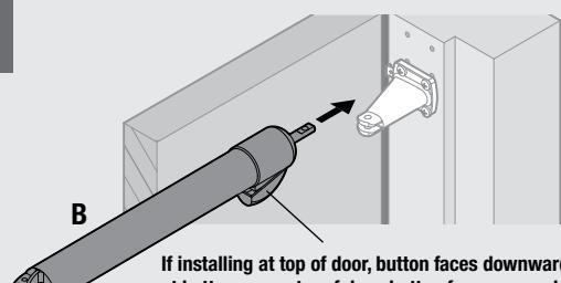
**If installing at top of door, button faces downward. If installing at bottom or center of door, button faces upward.**
