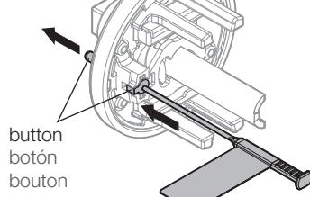
Rotate and remove spindle.
