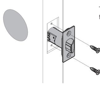
The slant of the latch bolt faces in the direction that the door closes.
