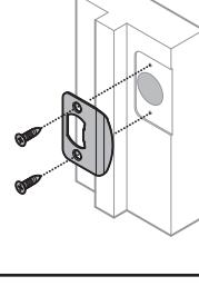
Close door and test latch operation. If latch is loose in the strike, adjust strike tab so it grips the latch bolt better when the door is closed.
