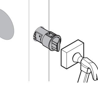
The slant of the latch bolt faces in the direction that the door closes.
