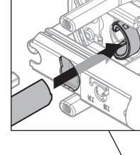
Align spindle with curved hole in latch.
