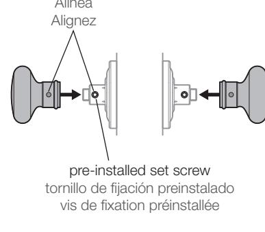
Tighten pre-installed set screws.
