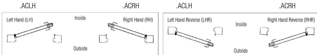
Handing determined by location of hinges. (LH) hinges are on the left & (RH) hinges are on the right.
