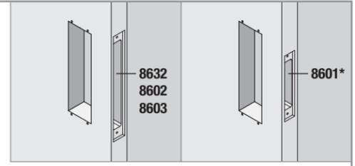
**\*If using a 8601 passage mortise, the trim plates may be positioned anywhere on the door, as the trim does not interact with the mortise box.**
