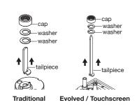
Install the cap and washer onto the new tailpiece, and place the assembly onto the cylinder. Press the pin down, and turn the cap clockwise to tighten. Once fully tightened, rotate the cap counterclockwise one notch.
