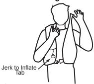
1. Inspect arming mechanism and cylinder if RED, service mechanism. Don like a jacket, with buckle centered in front, with 'Jerk to Inflate" handle at lower right.
