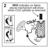
Push cylinder into housing and rotate 90° clockwise until it locks into place and **GREEN** indicator shows in window. The mechanism is now rearmed and ready for use.
