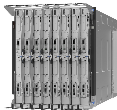
ThinkSystem N1380 Enclosure This Neptune® chassis is the core building block for the SC750 V4 and SC777 V4 servers and represents the next generation of Neptune® liquid cooling technology. The N1380 enables exascale-level performance while maintaining a standard 19-inch rack footprint. It is a 13U enclosure and supports 8 trays mounted vertically.
