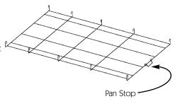
3 Locate the two Side Panels (C) and lay them flat on the floor, one on each lengthwise side of the Bottom Panel as shown. Lay the Side Panel with the Door on the right side of the Pan Stop. The loops on the short ends of each Side Panel and the exposed wires should face upward.
