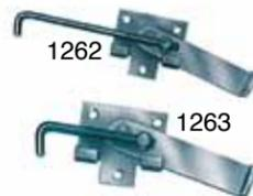
**1262/1263 Jamb Latches**—Cam action and adjustable hook holds door firmly against the jamb. 1262 has 7 in. hook; 1263 has 4 in. hook.
