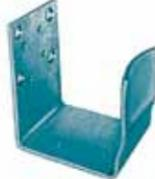
**325 Door Guides**—Extra wide guides ideal for corrugated metal-clad doors. Easy to install. Fasteners not furnished, but guides have holes for spikes as well as larger holes for ¾" lag-screw mounting. Guide is adjustable for doors 5" x 5½" thick. Curved section of guide may be turned sideways allowing straight access when installing screws.
