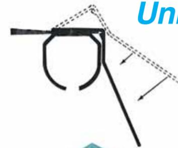
Simplifies rail installation. Just attach rail to track board and "snap-on" flashing brackets—then add flashing.
