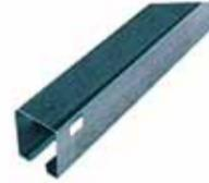
**6002 Door Laterals**—The galvanized 16 gauge laterals are pre-punched at each end for easy attaching to vertical members. All laterals have hanger holes pre-punched and can be used as either top, bottom or intermediate door members. Available in 4 to 20 ft. sections.
