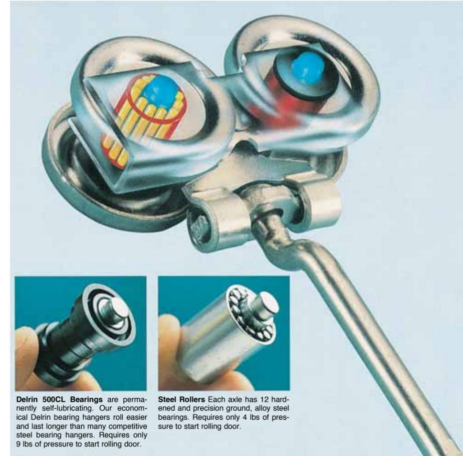
**Delrin 500CL Bearings** are permanently self-lubricating. Our economical Delrin bearing hangers roll easier and last longer than many competitive steel bearing hangers. Requires only 9 lbs of pressure to start rolling door.
