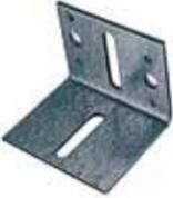
**6005 Guide Rail Bracket**—For use with No. 6004 Guide Rail. Slotted hole in each leg allows both lateral and vertical adjustments. Bolts, nuts and washers included.
