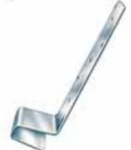
**6009 Jamb Mount Door Stop**—Stops and holds door in both open and closed positions. The end with right angle projects slightly beyond the jamb and engages the vertical member of TAB-LOC™ or EASY-FRAME® door frame. Available in 3 sizes.
