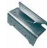
**6007W Center Guide**—For use in pairs. The 6007W is a heavy-duty center guide for single or bi-parting MAX EASY-FRAME® doors and is recommended for single doors 16 foot and wider, plus all bi-parting MAX EASY-FRAME® door systems. Should be installed in the center of the opening and works with the 6053 bottom lateral.
