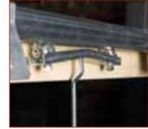
Tandem brackets double the capacity of the rail on larger door applications. Heavy doors roll smoother with the tandem bracket without the need for a center-mounted trolley hanger.
