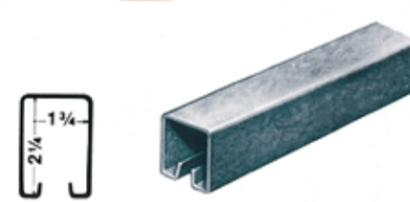
**No. 5116 Rail**—For doors weighing up to 450 lbs. per panel. 16 gauge galvanized steel rail bundled without fasteners or brackets. Can be used with various types of single and multiple brackets.
