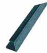
**6004 Guide Rail**—Engages the bottom lateral of TAB-LOC™ doors to hold the door in place and prevent wind damage. Fastens to building with No. 6005 Guide Rail Bracket. Guide rail also used with 6061/6062 Continuous Bottom Guides.
