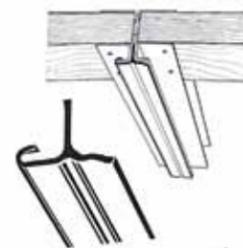
**6027 Door Astragal**—A prefinished, white, extruded aluminum used to cover the gap between bi-parting doors. The unique design allows it to wrap around the flashing channel of the vertical. Astragal fits both TAB-LOC™ and EASY-FRAME® doors and attaches with pop rivets. Available in 10, 12, 14, and 16 foot lengths.
