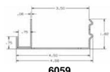
**6061 1 1/2" Continuous Bottom Guide**—For use on wood frame doors. When nailed to the bottom of a 1 1/2" wood framed door, the continuous bottom guide engages with the No. 6004 Guide Rail to prevent damage to door or building.
