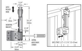
When used in a swimming pool or spa application, the Vertical Pull model should be used on gates that are 5 feet (1524mm) or higher.
