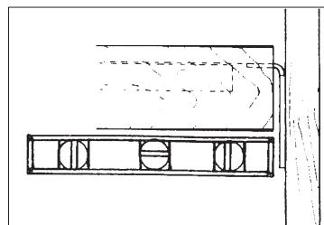
Level the Header Assembly at the correct height and nail End Bracket to Jamb.
