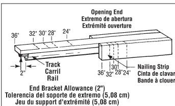
**NOTE:** Header assembly premarked Door width. Header markings accommodate inside Trim of Pocket.
