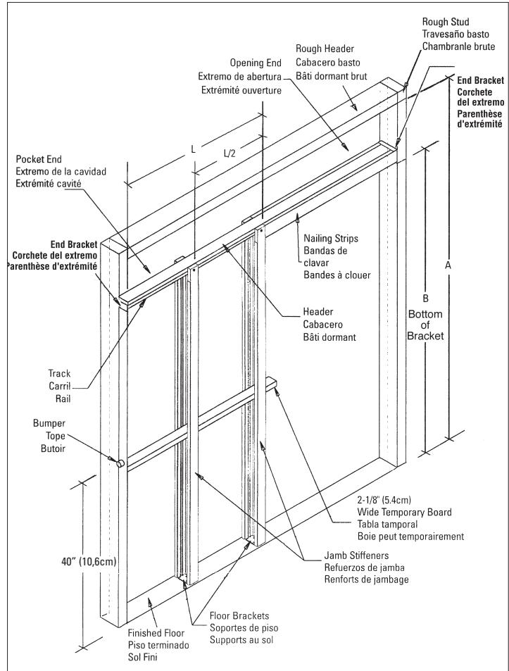
Prepare rough opening. Finished Floor to Rough Header height should be minimum of (A) See Table and Figure 1. Determine width of rough opening by multiplying door width by 2 and adding 1-1/4" (31,8 mm).
