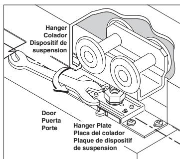
Using the Wrench supplied, turn the adjustment Post so that the Door is Plumb and has proper floor clearance.
