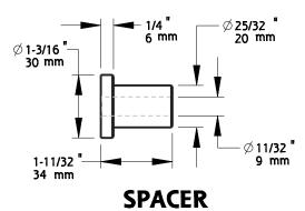
Fasteners: (4) Hex Screw, M8 x 3-1/2" Long (4) Hole Cap (4) Washer, M8 (4) Spacer
