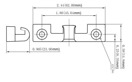
1.Material: Aluminum or zinc cast zinc die cast 2.Supplied with(4) #7×3/4" steel. Full thread,oval head, recess. Hardened, wood screw
