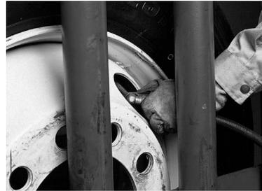
5. Inflate assembly to set bead and check for leaks around the wheel.
