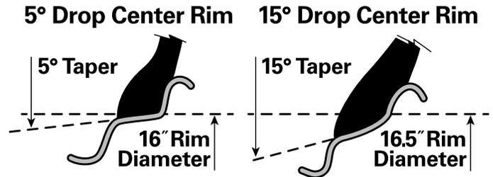
The following diagram shows how the beads of a 16" tire will not seat on a 16.5" rim. The beads should not be forced out against the rim flanges by using more air pressure, because this will break the beads and the tire will explode. Never exceed 40 psi when seating the beads on the rims.
