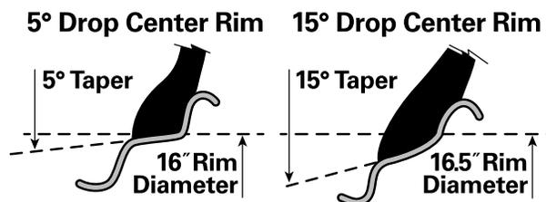
The following diagram shows how the beads of a 16" tire will not seat on a 16.5" rim. The beads cannot be forced out against the rim flanges by using more air pressure, because this will break the beads and the tire will explode.
