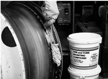
3. Lubricate the wheel bead seat using vegetable oil-based lubricant approved for both tire and wheel.
