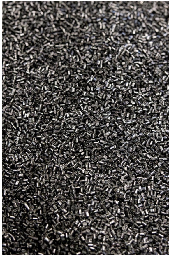
Pelletized recycled high-impact polystyrene (HIPS), ready for reuse (Source: Canon Virginia, Inc.).
