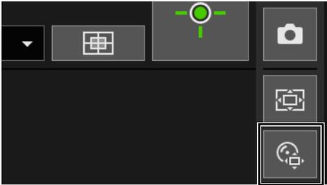
The [Digital PTZ] button changes active (purple), and the Digital PTZ panel is shown in the control display area.
