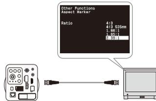
Since the camera is directly connected to the external monitor, you can adjust images on the screen by directly operating the camera.
