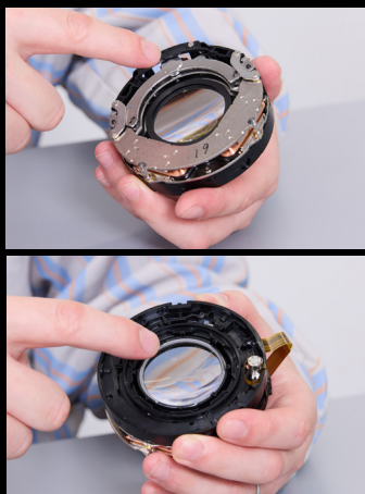
A newly developed actuator responsively controls Image Stabilizer optics.
