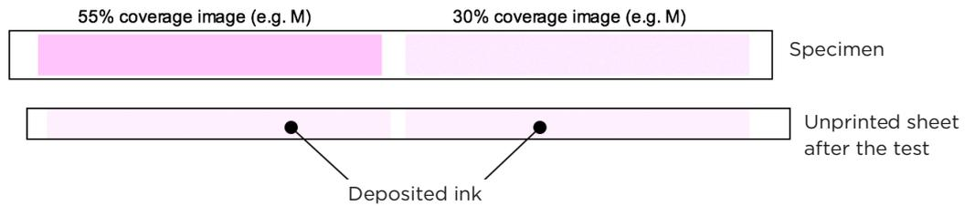
The optical density of the ink deposited on/transferred to the unprinted sheet was measured with a spectrophotometer. The optical density is the measure for surface tack/smudge. An optical density smaller than 0.025 (i.e. hardly any transfer of ink) is considered to be sufficient to ensure post-processing and handling of the medium without risk of distortion of the image or smudging of the medium's rear surface on the winder.
