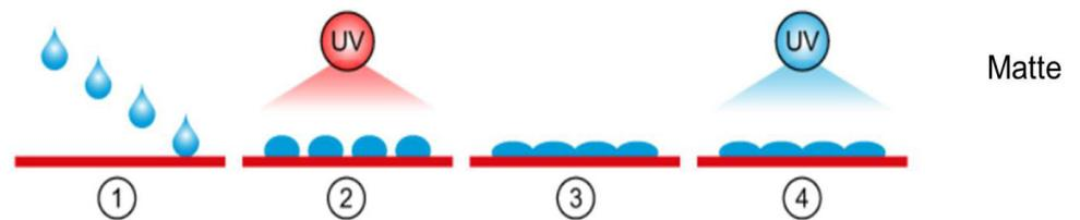
Similar to creating a gloss print, the unprinted media is transported under the printhead head carriage, where the image is being built up by jetting the gel droplets onto the substrate. In contrast to printing in gloss mode, that wet ink layer is being flashed intermediately with a low dose of LED UV-light.
