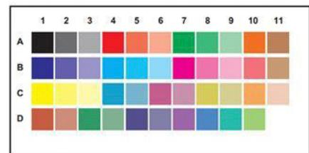
The test target was measured at regular intervals using a spectrophotometer. From this data the color difference in dE was charted and judged on the visibility of color change (dE00) after 2700 hours.
