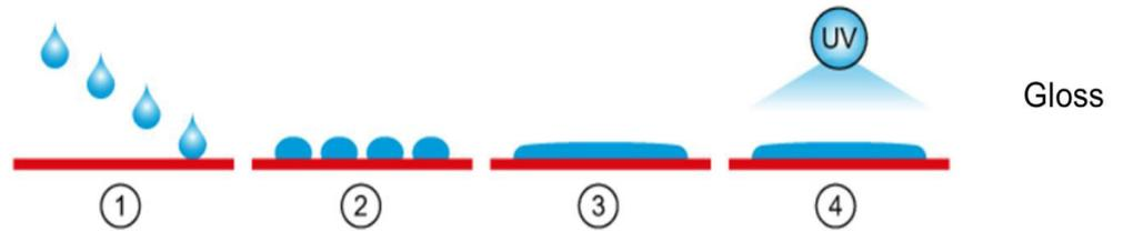
First, the media is transported under the printhead carriage, where the ink is jetted onto the media and the image formed. At this stage, no curing energy reaches the ink and the image is completely being built up while the ink and image remains completely uncured.
