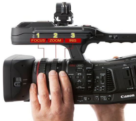
Figure 3 The 18-element lens that comprises 14 groups – and the three control rings for separate zoom, focus, and iris control
