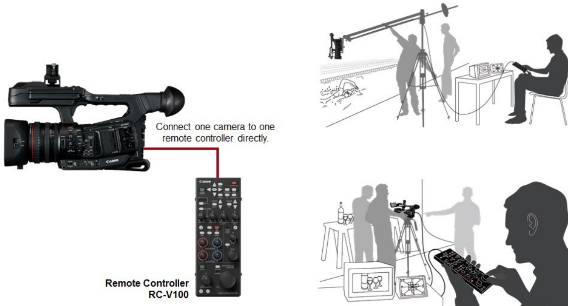
Figure 32 Canon remote controller RC-V100 connects directly to the XF705 camcorder
