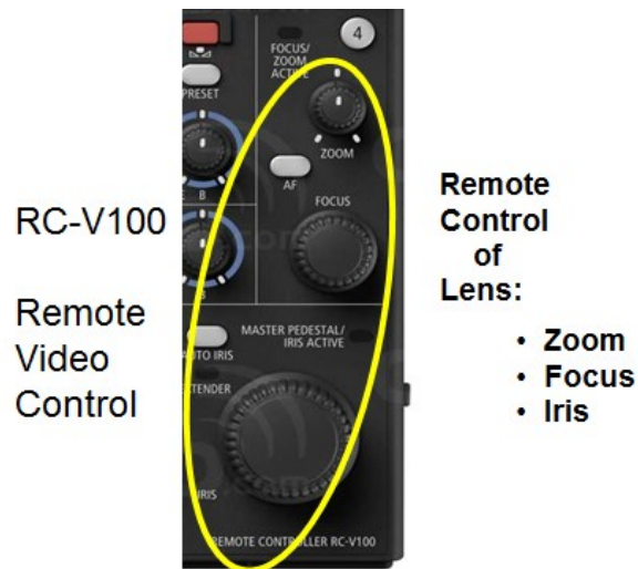
Figure 33 The lens zoom, focus, and iris can all be remotely controlled from the RC-V100
