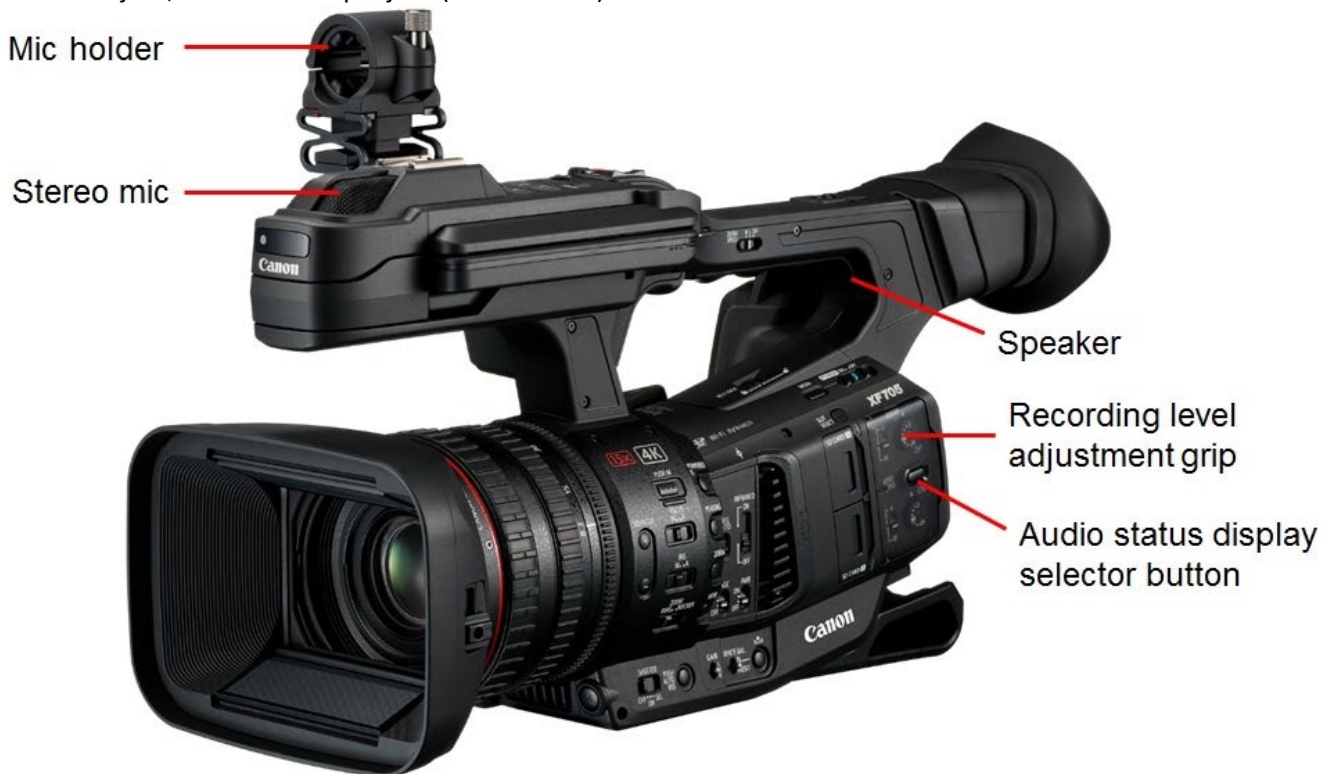
Figure 25 Identifying the audio interfaces in the XF705
