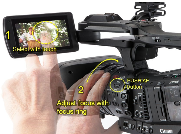
Figure 9 The LCD monitor is a capacitive touch screen that supports movement of the focus frame (including magnification)
