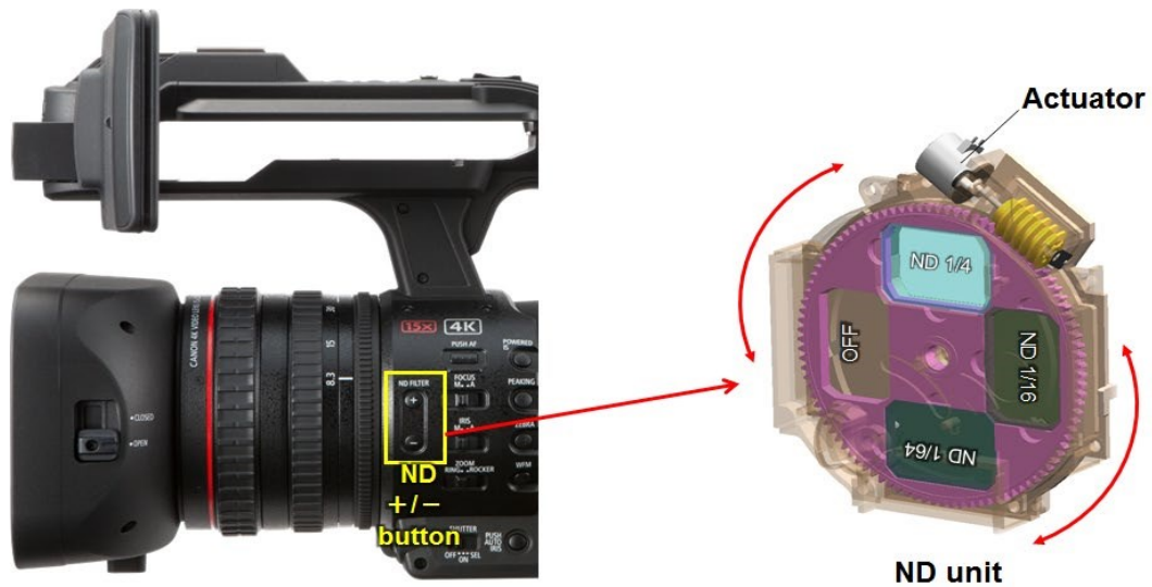
Figure 7 Showing the internal turret mechanism used to select one of three ND filters in XF705
