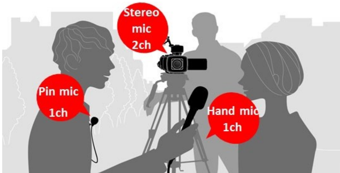
Figure 26 Identifying the potential use of the four audio channels in XF705
