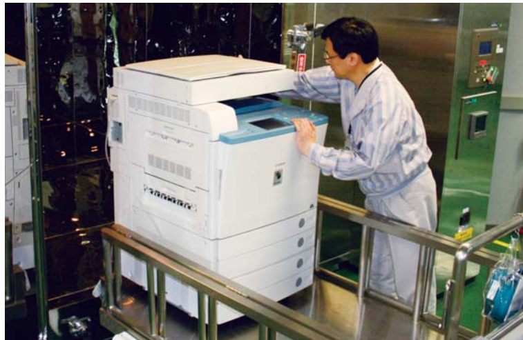
Measuring chemical substances released from a digital MFP
