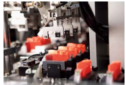
Automated production of ink tanks
