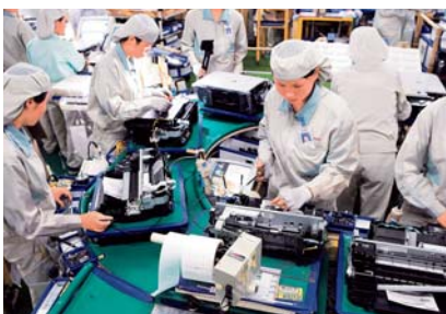
Introducing the cell production system in which an individual worker performs multiple processes
