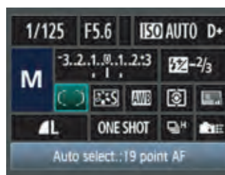
The Quick Settings screen, which enables the user to configure and customize photographic parameters intuitively
