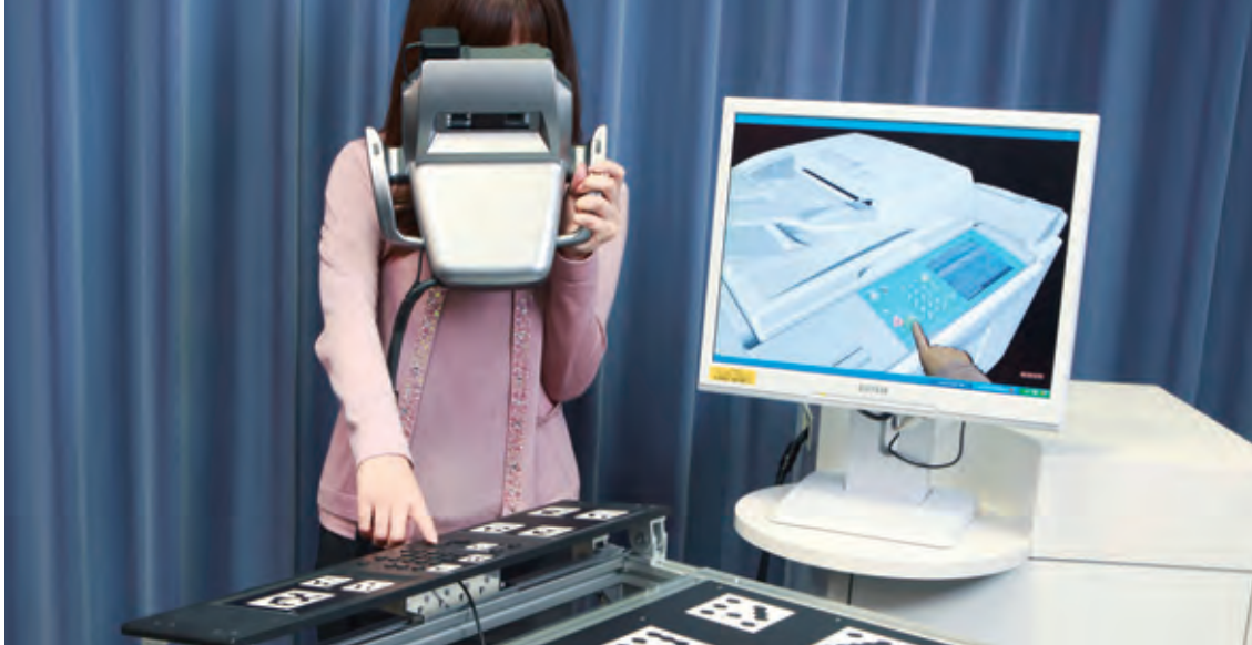
Simulation of office network MFD operation using MR technology (The display screen image is also depicted on the HMD.)
