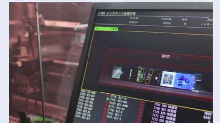
Canon Automated Recycling System for Ink Cartridges (CARS-I): camera-based technology used for automatic sorting of post-use ink cartridges
