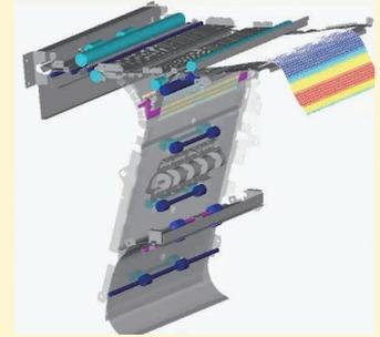
Simulation of paper feeding process inside a printer
