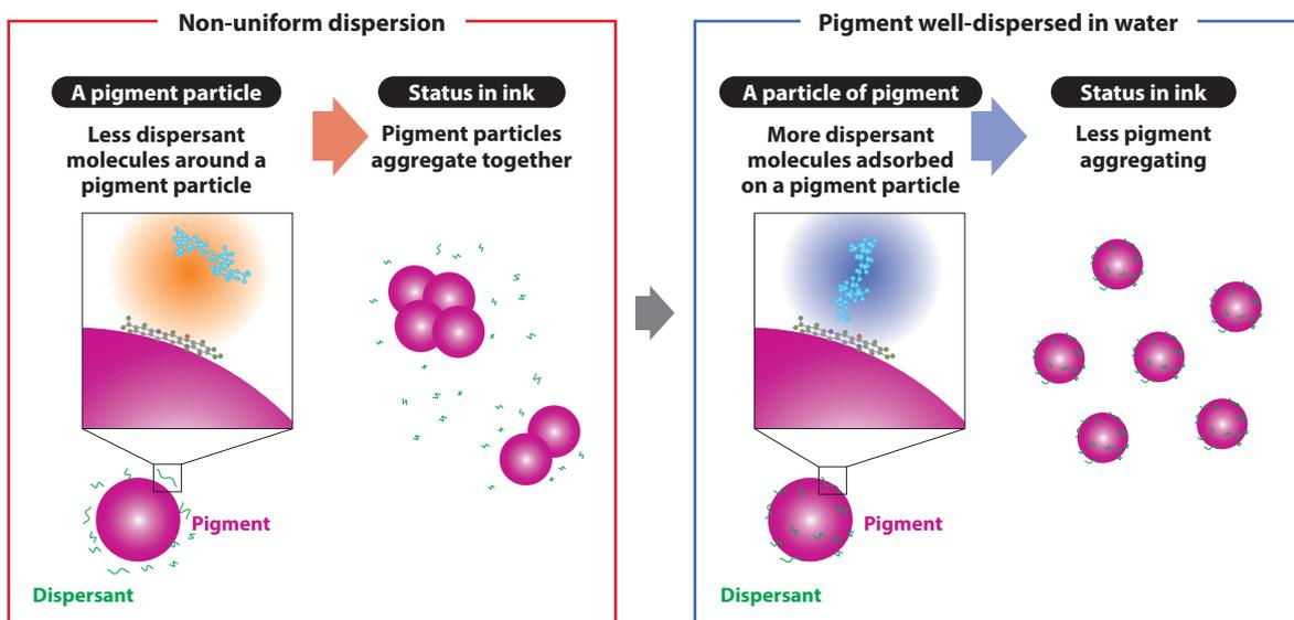
Finding optimal molecular structure of pigment and dispersant to secure uniform dispersion
