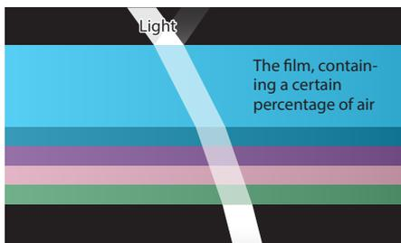
The film, containing a certain percentage of air with lower refractive index than optical glass, forms an ultra-low refractive index layer
