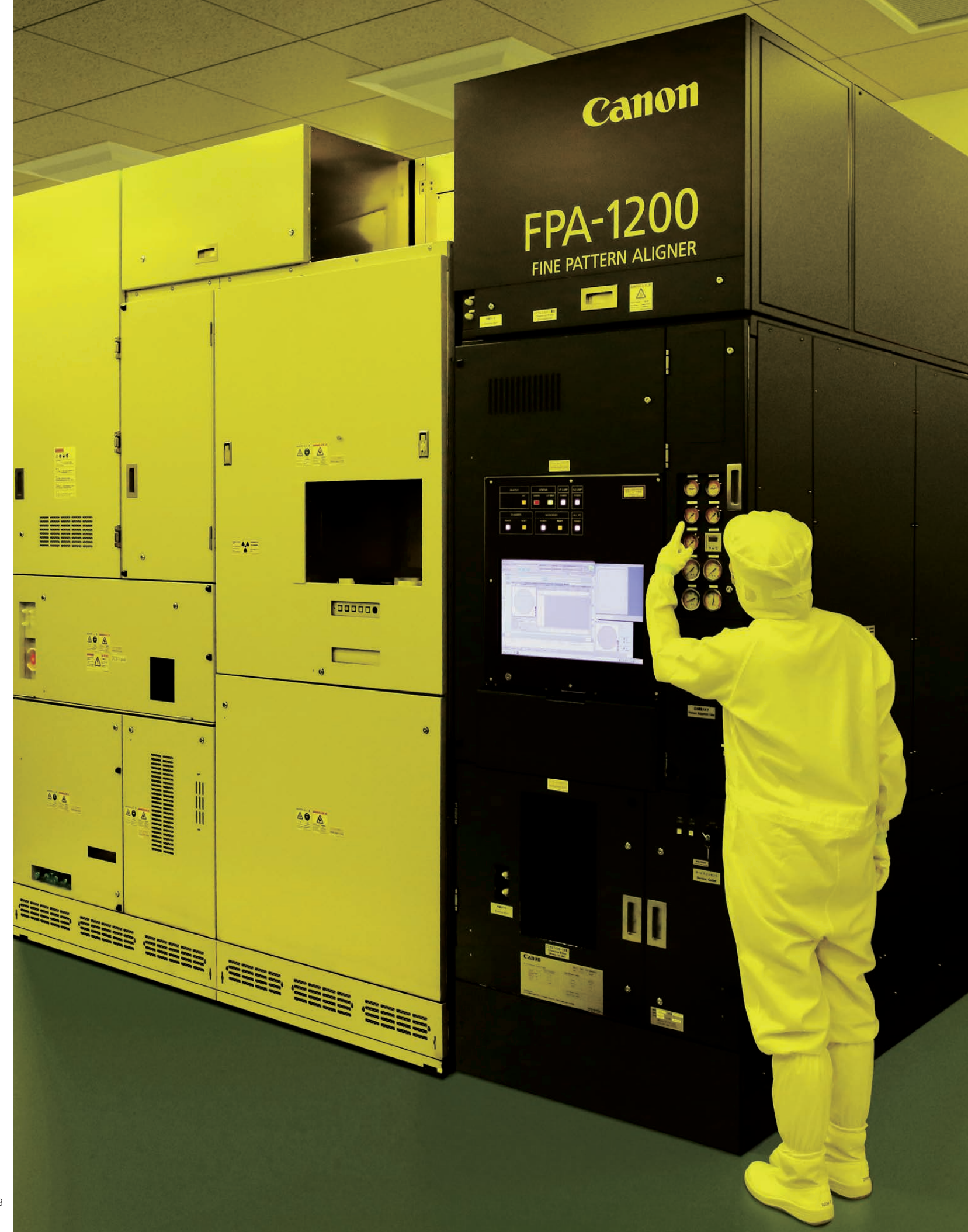
The FPA-1200N22C nanoimprint semiconductor manufacturing system launched in October 2023
