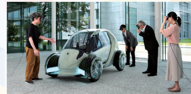
Life-size CG images can be displayed in a real-world environment viewed through a HMD
