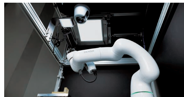
A network camera watches over a quality inspection process
