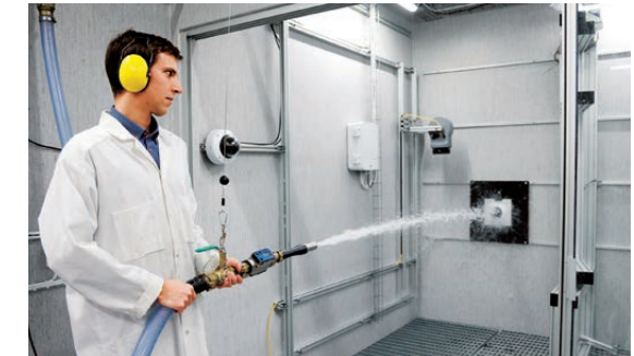
Testing the durability of network cameras at Axis
