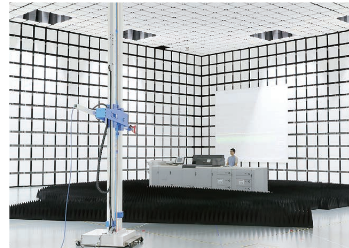
Quality tests on a digital commercial printer performed in an anechoic chamber that is not affected by electromagnetic interference
