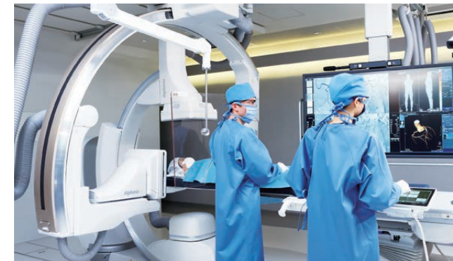
X-ray angiography system that uses X-rays to visualize the condition of vessels in real-time
