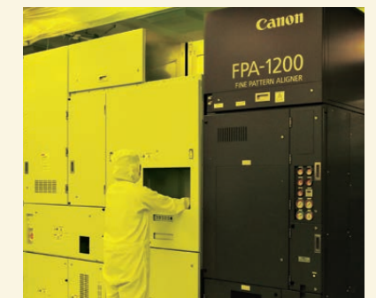
Canon's nanoimprint semiconductor production equipment
