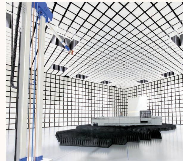
Quality tests on a digital commercial printer performed in an anechoic chamber that is not affected by electromagnetic interference
