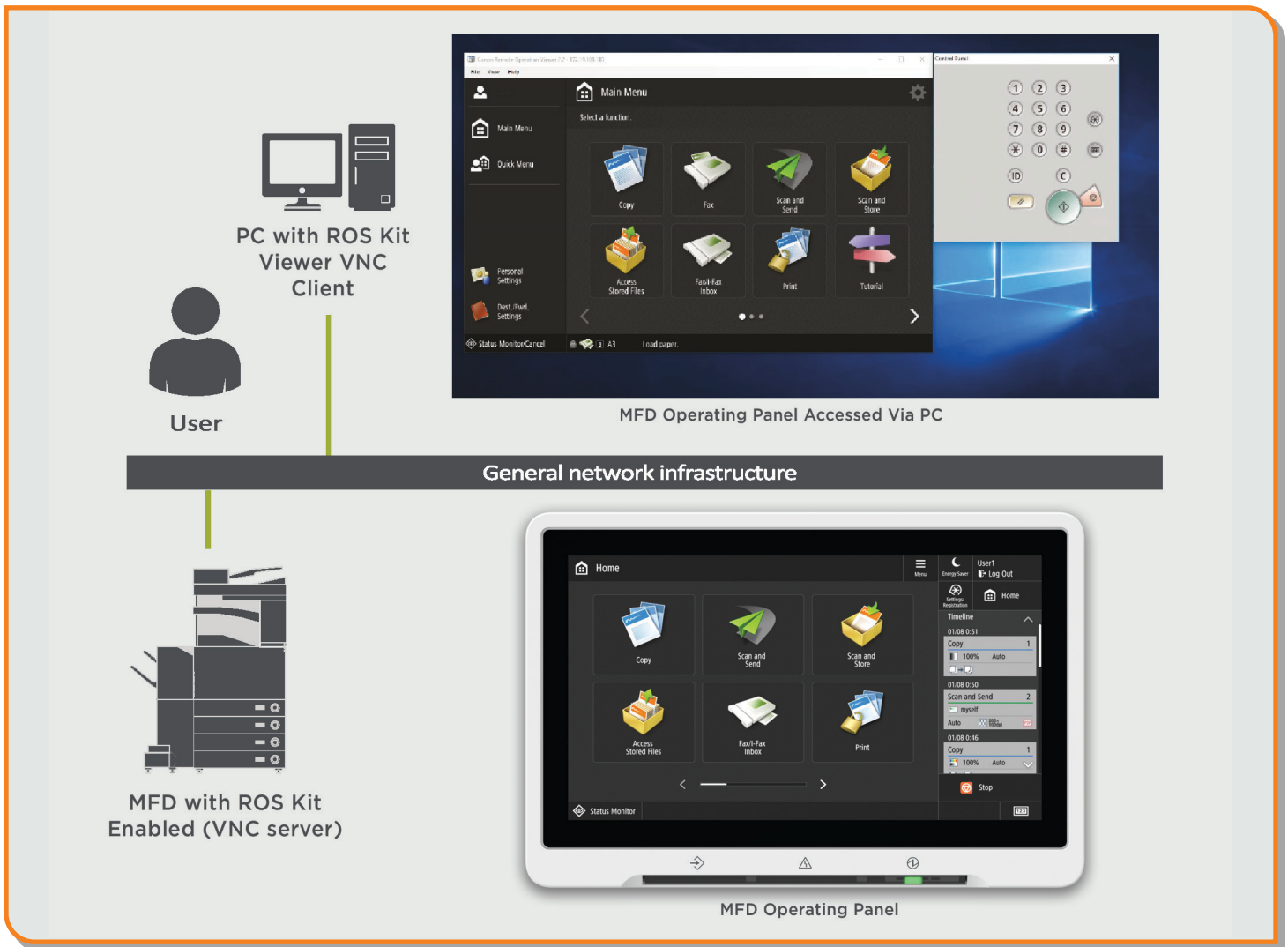
Figure 14: Remote Operator's Software Kit (ROS Kit) Setup
