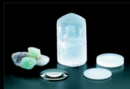
Raw fluorite crystals, artificial fluorite crystals and fluorite lenses
