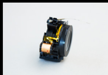
Focus lens unit driven by VCM
