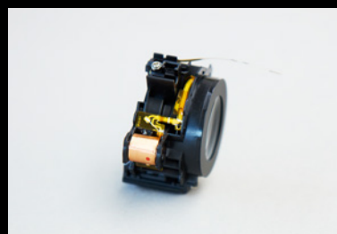
Focus lens unit driven by VCM
