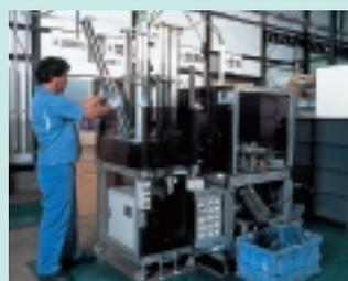
Automatic disassembly equipment for Bubble Jet ink cartridges
