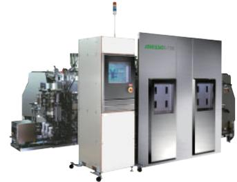
Sputtering equipment used to manufacture super high density HDD magnetic heads
