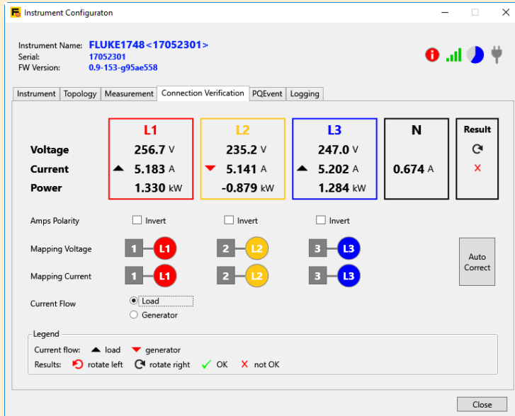
Connection verification function shows whether the instrument is connected correctly and automatically corrects issues at the press of a button.
